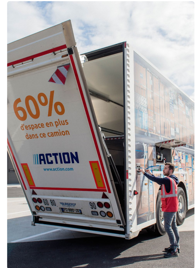
Our double-decker trailers enable us to carry 60% more freight per truck. Fewer transport trips mean lower fuel usage and lower emissions.
