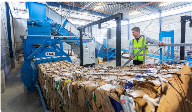
A new massive bale press helps reducing the volume of cardboard and plastic packaging waste, making it ready for a more CO 2 efficient transport to recycling facilities.
